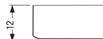
Detail Z Q1 and Q2 - square face 90° turn-up for installation in square tile ceilings
